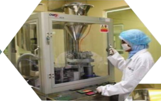
Capsule Filling Machine (15,000 pieces/hour)
