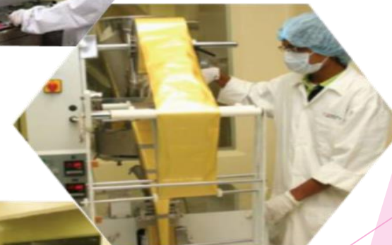
Capsule Filling Machine (15,000 pieces/hour)
