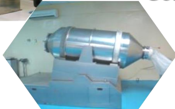
Two-Dimensional Mixer (400kg/batch)
